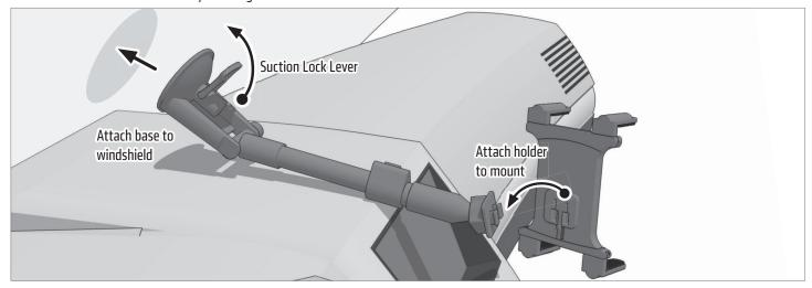
2 Adjust length of mount as necessary by unlocking extension arm. Lock arm when desired length reached. Insert device by pushing down on lower legs of spring-loaded holder.
