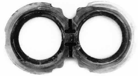
Wearplate showing the effects of overheating
