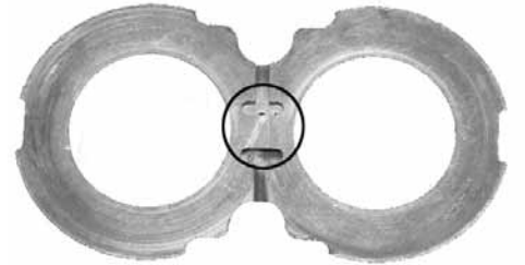
Jetting caused by fine particle contamination
