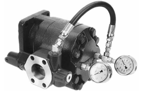
Pumps which are designed to easily accommodate vacuum and pressure gauges save maintenance time and provide greater accuracy. The special rear test ports shown in this view of the Muncie Power-Pro may be used for monitoring performance. The birotational four-port pumps (K & L Series) are also very accessible for gauge installations.
