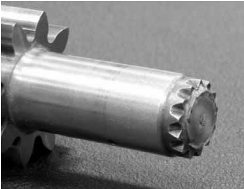
This pump shaft was twisted off due to a sudden pressure spike.
