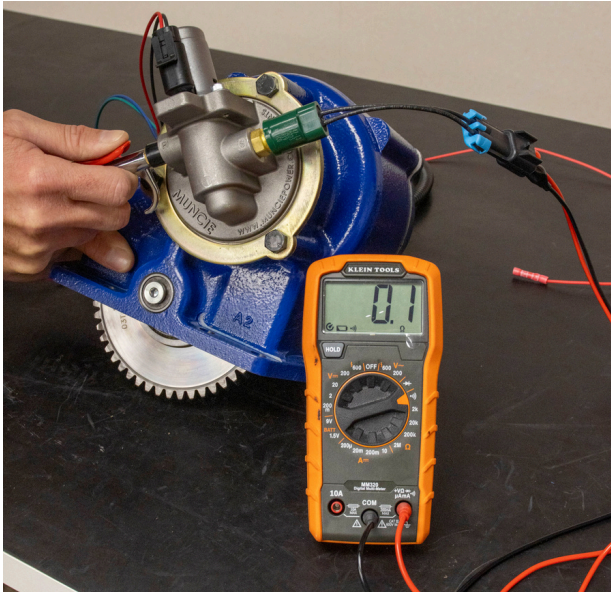
Figure 3. Testing pressure switch for continuity when PTO is engaged.
