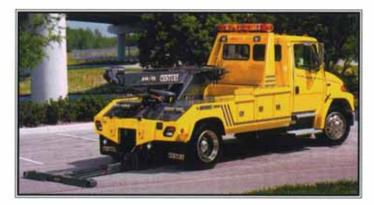
The Formula II T underlift is constructed using a fabricated inner stinger for added strength while still maintaining a low profile. The twin tilt cylinders provide a total range of 22° positive and negative tilt.
