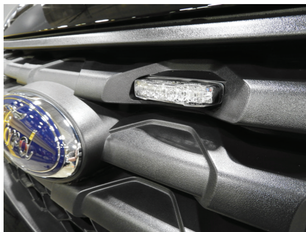
MicroPulse C Series shown mounted in grille
