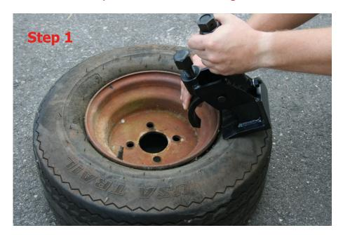
1. Place bead breaker onto the rim with teeth and breaker foot between rim & tire bead.
