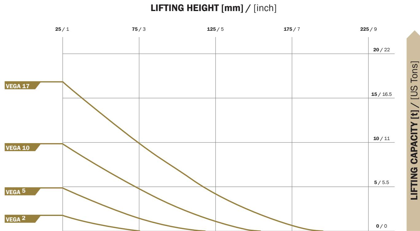
**Graph 5: Lifting capacity of high-pressure lifting bags SLK**
