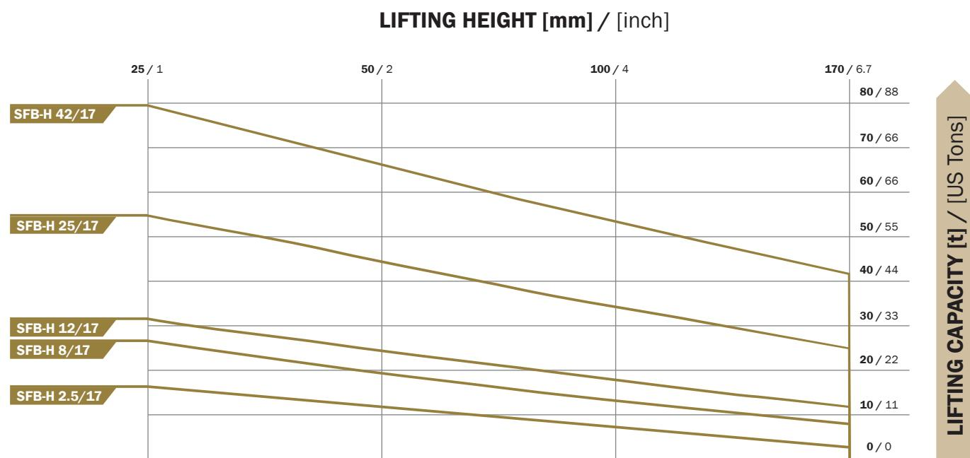
**Graph 10: Lifting capacity of high-pressure lifting bags Flat+**
