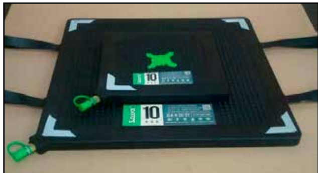
Fig. 5.27: Combining SAVA conventional lifting bags to increase the lifting height
