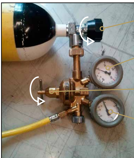
Fig. 5.7: Set pressure reducing valve
