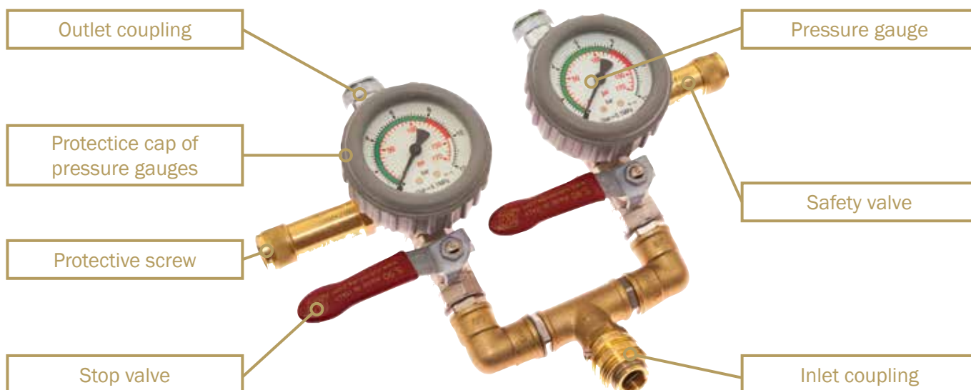
Fig. 6.7: Fitting controller
