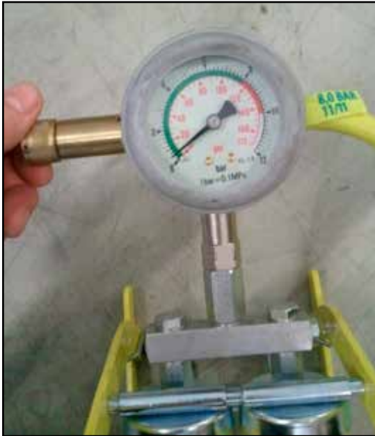
Fig. 5.15: Tightening or unscrewing the protective screw on the safety valve of foot pump
