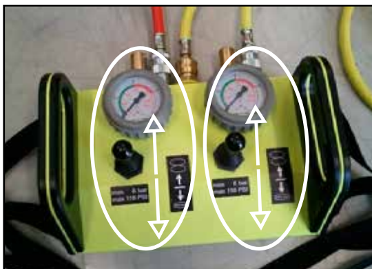
Fig. 5.10: Dual deadman controller - metallic
