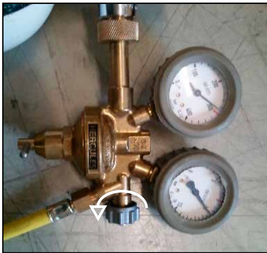
Fig. 5.9: Relieve the pressure reducing valve
