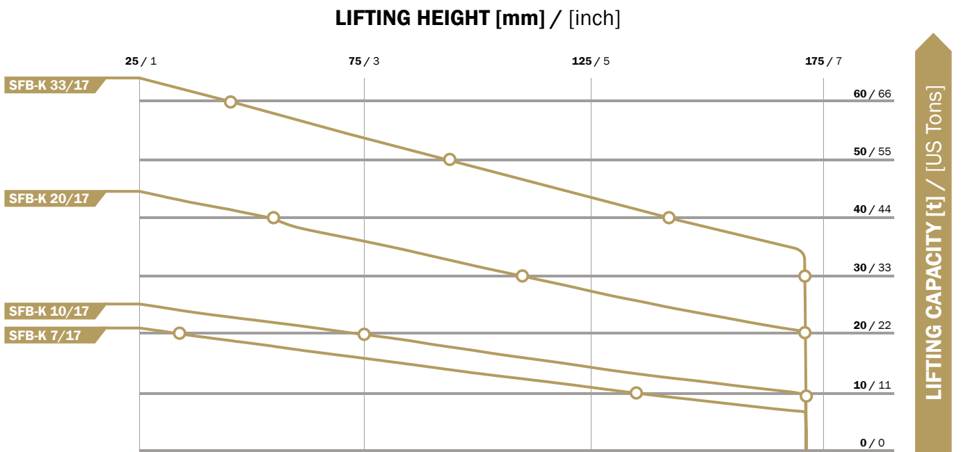
Fig. 2.6: Maximum lifting capacity of FLAT BAG SAVA SFB-K lifting bag, depending on the lifting height
