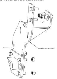
**5.** Mount the **PUSHBAR** (1) in place between the two side plates using eight ½"-13x1-1/2" **BOLTS** (5) and eight ½"-13 **LOCK NUTS** (8). The centerline of the Pushbar Crosspin should be approximately 9-1/2" from the ground. The air dam of the vehicle may need to be altered to accommodate this height. Improper mounting height will result in uneven cutting edge wear.
