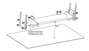
**6.** Install the Center Bracket onto the push bar (loosely) with four  $\frac{1}{2}$ " Bolts and Nuts (5&8). Toward the rear of the bracket, choose two of four holes to install onto the cross-frame. Secure it onto the cross-frame of the truck with two bolts-stick (6) and two nuts (9) with two washers.
