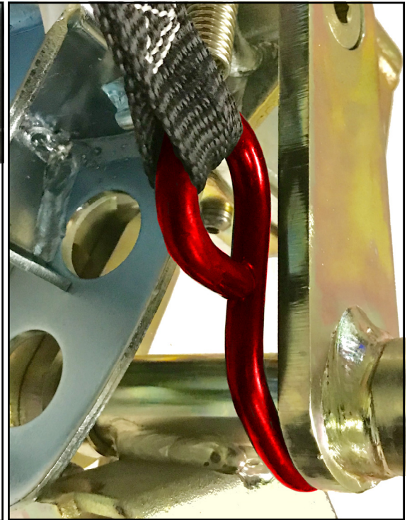
Hook Around Bottom of Spindle
