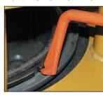
• Separator end Separates split ring from solid flange ring to form gap
