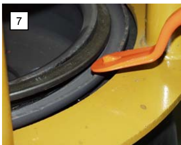
Start demounting the raised end of the split ring by placing the end of the tip of the DEMOUNT end under the split ring.
