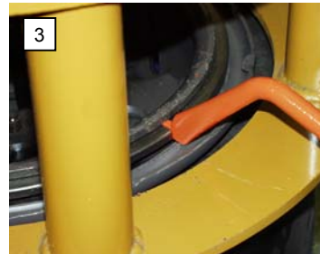
Push down to separate the solid ring from the split ring.
