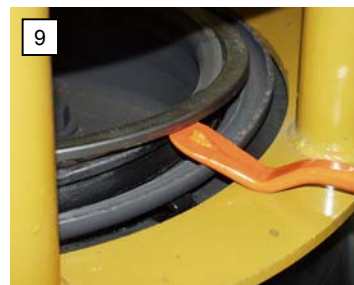
Push down to pry up, working around the ring until it is demounted.
