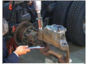
FIGURE 71 - REMOVE THE LONG GUIDE PIN
