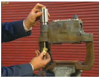
FIGURE 70 - INSTALL THE REMOVAL TOOL
