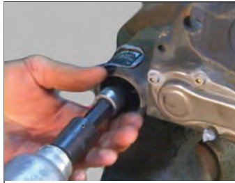
FIGURE 67 - REMOVE THE CALIPER BOLTS
